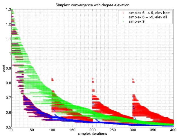
3 simplex optimizations with Bezier parametrization in chordwise direction of different degrees:
