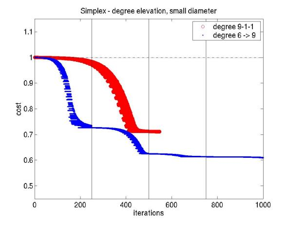
2 simplex optimizations with Bezier parametrization in chordwise direction of different degrees:
