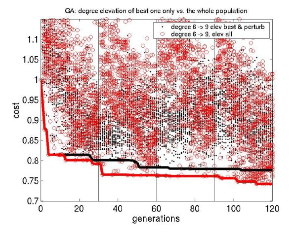
2 GA optimizations with Bezier degree elevation, the same parametrization, difference in inheriting information at elevation process:
