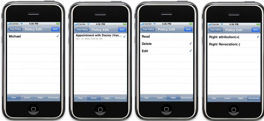
Figure 6. Selection of various attributes to insert a new rule in policy in iPhone OS implementation
