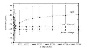
(a) Inefficiency ratio as a function of the object size; FEC expansion ratio = 1.5
