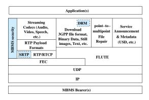
Figure 7: The MBMS protocol stack in the downlink.
