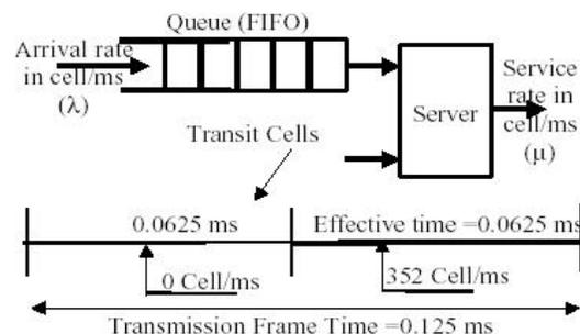
Figure 2 Queue Model for ADM/ATM Node
