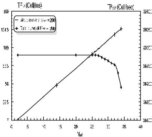
Figure 7  $TP_{vi}$  &  $TP_{da}$  versus  $N_{vi}$  with  $R_{vi} = 1.5$  Mbps, and  $\mu = 5$  ms.
