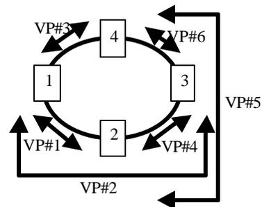
Figure 1 VP-Based ATM Ring network.
