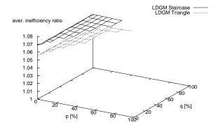
(d) LDGM Triangle vs. Staircase and a FEC expansion ratio of 1.5.
