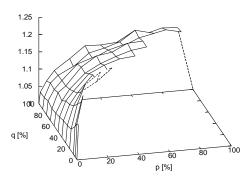
(a) RSE and a FEC expansion ratio of 2.5 (NB: the figure is rotated for better visibility).
