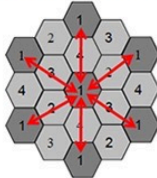
Increased Frequency Reuse (w/ 80 MHz channels) - All same-channel BSS blocking
