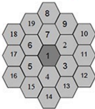
Low Frequency Reuse (w/ 20 MHz channels)
