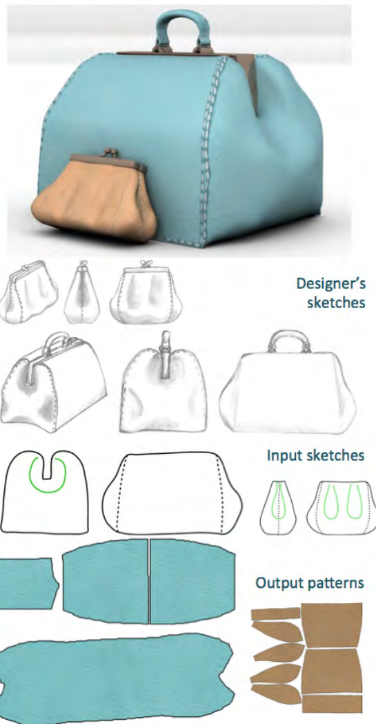
Fig. 15. Top: Doctor bag and leather purse designed with our system. Middle: designer's sketches exhibiting design folds which are intended to remain permanently on the product and the sketches given as input to our system. Bottom: the patterns we output. Note that we did not use symmetry for these examples: therefore, neither the input sketches nor the resulting shapes or patterns are fully symmetric.
