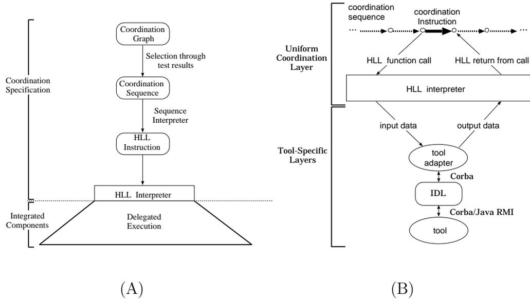
Fig. 4. The Coordination Environment in the ITE Scenario
