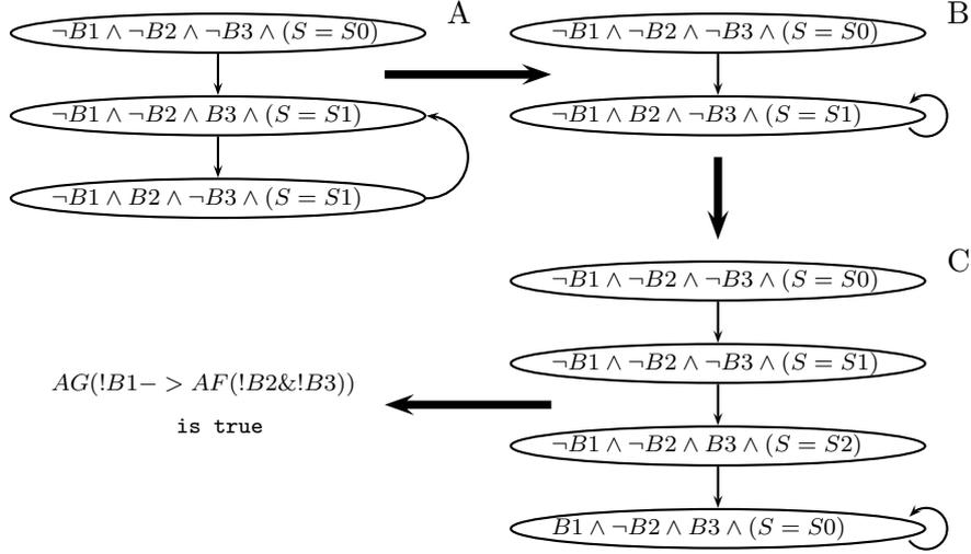
Fig. 4. Error traces generated by model checking different levels of refinement
