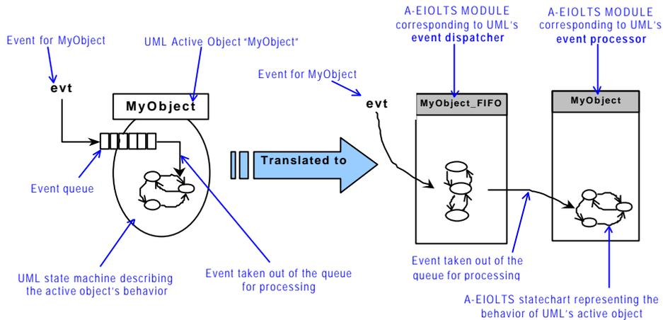
Fig. 4 – Decomposition of a UML active object into two A-EIOLTS modules
