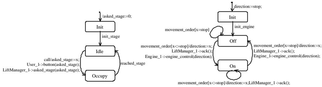
Fig.11 - State machines for the stage recorder (left) and the engine manager (right)
