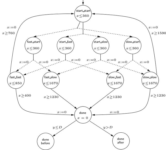
Fig. 3. Probabilistic timed automaton  $I_1^p$  modelling the root contention protocol.
