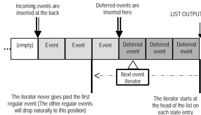
Fig.8 – Theoretical implementation of a FIFO with improved deferred event handling
