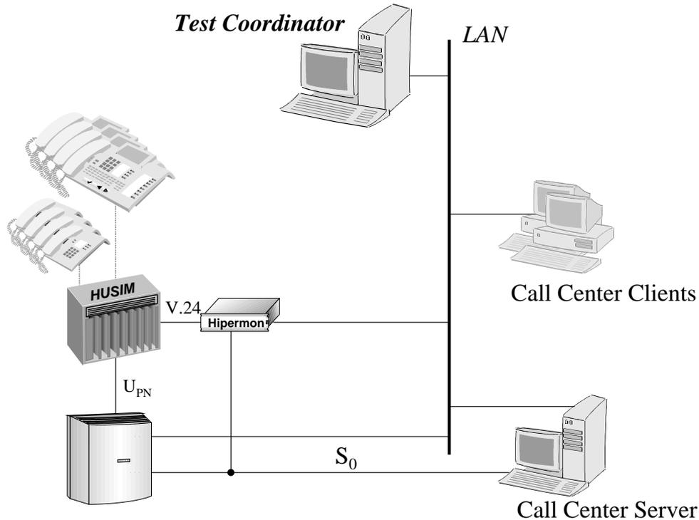
Fig. 1. Example of an Integrated CTI Platform
