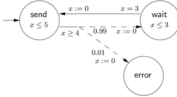
Fig. 1. An example of a probabilistic timed automaton  $\text{PTA}_1$ .
