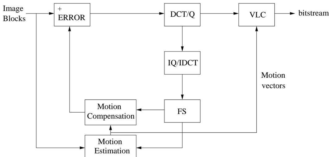
Fig. 2. Block diagram of the MPEG-2
