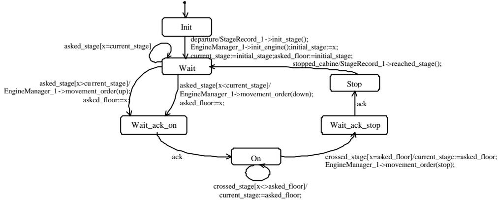
Fig.12 – State machine of the lift manager
